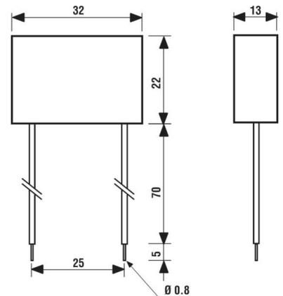
[Capacitor 1  \$\mu\$ F 230 V Parallel capacitor for L-lamp 02600 online kaufen](#)
